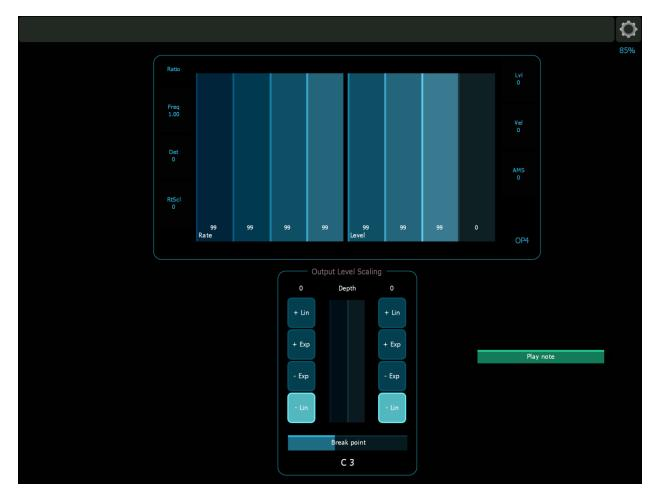
Output Level Scaling can be adjusted using the preset curves and breakpoint. I do not plan on implementing Fractional scaling at this time. When you are finished, press the Operator name again to close this display.
