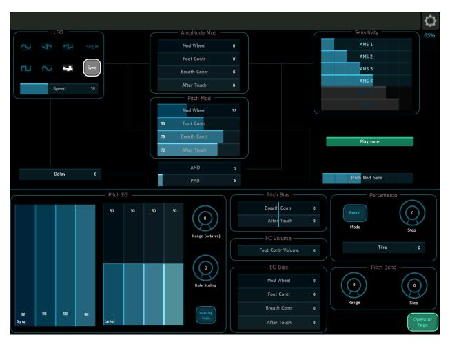
Most controls are self-explanatory. Sliders with a value embedded in them will automatically move the value to the other side as you change the slider position. This allows you to always see the current value.
