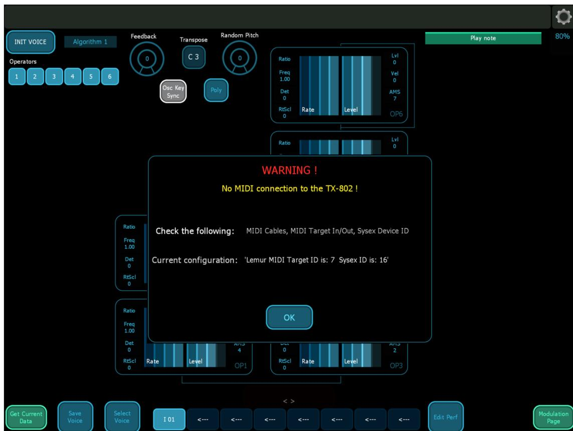
At this point, clear the error, go back into the Configuration menu and verify the settings. If the settings look good, verify the Lemur port connections using the Lemur control, select 'More settings...', and then reselect the appropriate MIDI connection for the ports. Exit the Lemur menu and press the Get Current Data button again. To preserve your settings, use the Lemur control and choose Save Project...
