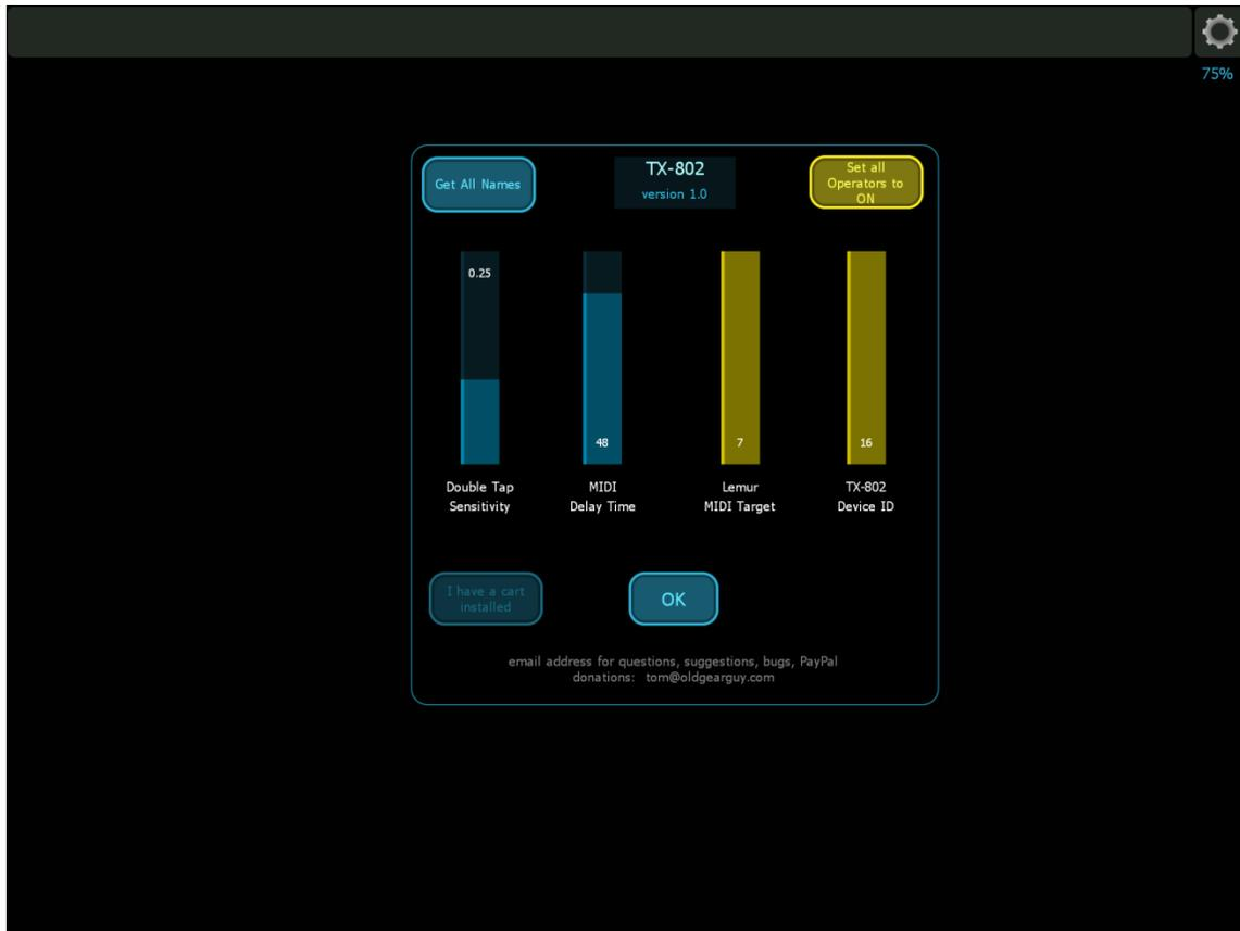
Set the Lemur MIDI Target and TX-802 Device ID to match your system. Then press the Set all Operators to ON button. The sliders and button should revert back to their normal color. The 'Get All Names' button is not implemented yet.
