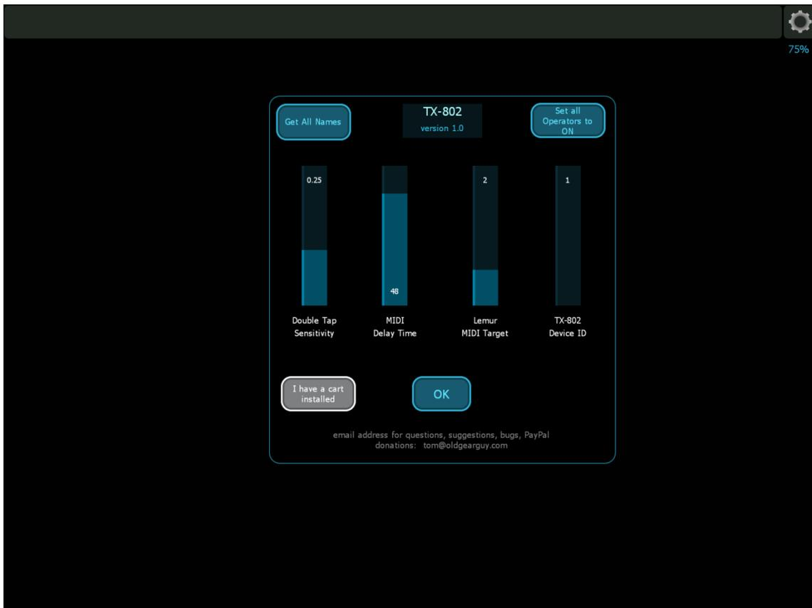
Press OK and exit back to the main screen. If the TX-802 is connected properly, pressing the Get Current Data button in the lower left corner will cause the editor to pull back the current Performance and Voices. While the transfer is happening, the Performance section on the bottom will flash blue. Once the flashing stops and the color reverts to normal, you can begin.
